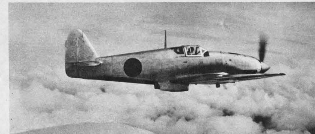
BULLET NOSE and faired cockpit distinguish Tony from Judy (top left). Other important features are the humped fuselage, the prominent belly radiator and the rudder's almost vertical trailing edge.
